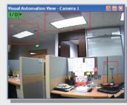
Visual Automation can be used to operate electronic appliances by triggering the output device. This means that you can control an appliance (e.g. Light On / Off; Door Open / Close) by simply clicking its image on the monitor.
