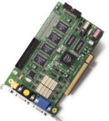
PCI Dsub - Type 170 (W) x 95 (H) mm
